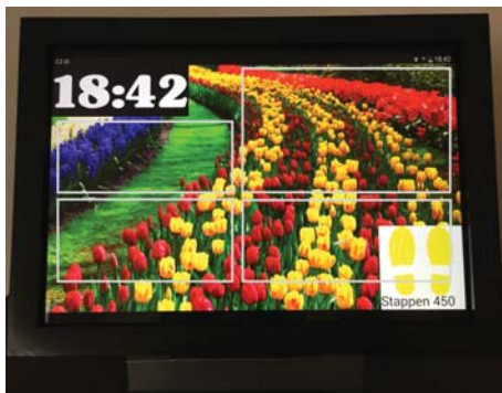
Figure 5: The implemented Android app on MyHealthFrame tablet is always running and cannot be closed.
